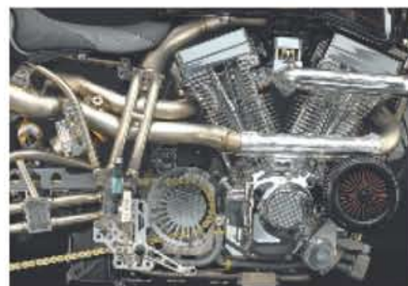
The engine is machined from a single block of aluminium
